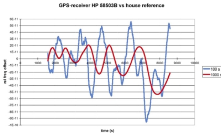
Figure 4. Frequency variation of a GPS-disciplined OCXO over an observation period of some hours. The average output frequency over 100s intervals varies from -1 \cdot 10^{-10} to +6 \cdot 10^{-11} . Measurements performed at Pendulum Instruments.
